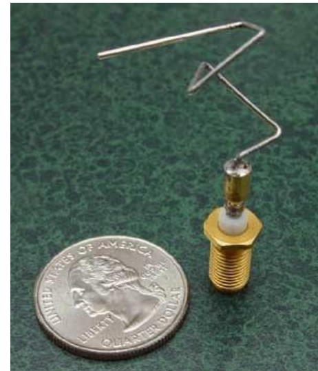
The NASA ST5 spacecraft antenna evolved by GP
