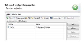
According to documentation the variable PATH must be set up.
