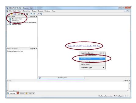
b. After iMpact verifies that the cable is connected it will prompt you to load your .bit file that you generated in step 6. Note that this file selection window doesn't always default to your existing project so you may need to navigate to your project folder and locate the .bit file. This file is always named to your top module so in our case it is simple\_verilog.bit. Double-click or select the bit file and click open, again make sure it is the right file.
