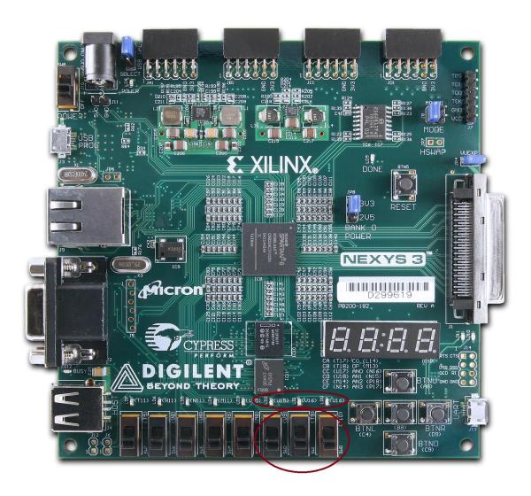
**UCF** (**User Constraints File**): Because we're headed towards putting this on the Xilinx FPGA on the Nexys 3 board, we need to set some constraints. In particular, we need to tell ISE which pins on the Xilinx chip we want **A**, **B**, **C**, and **F** assigned to so that we can access those from switches and LEDs on the Nexys 3 board. For that we need a "User Constraints File".
