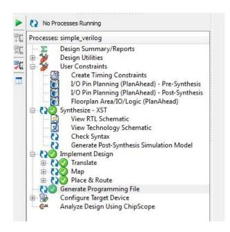
**Attention:** Before proceeding to the next step connect the board via the USB cable to the PC you're using, and turn on the power, the next step ensure proper connection to the board. Also note that you do not have to do steps 4, 5, and 6 individually. These processes are dependent on each other, if one needs a preceding process to be updated then it will automatically run that process before it runs itself. So you can just proceed to step 7 and watch ISE do everything.
