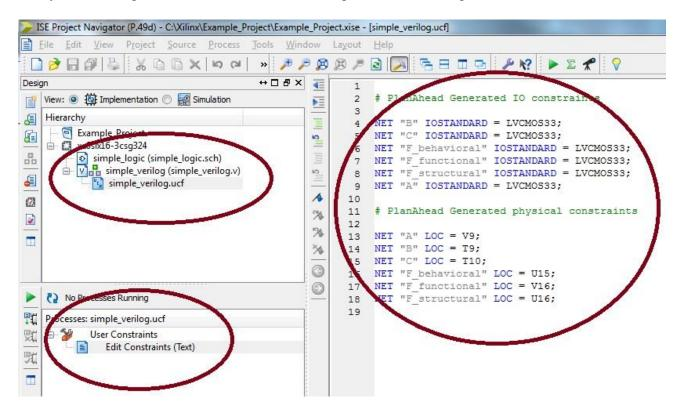
After you're done changing every port to LVCMOS33 and putting the right Pin # for all the ports in the design, click the **SAVE** button from the top menu in the page and close down Plan Ahead.
