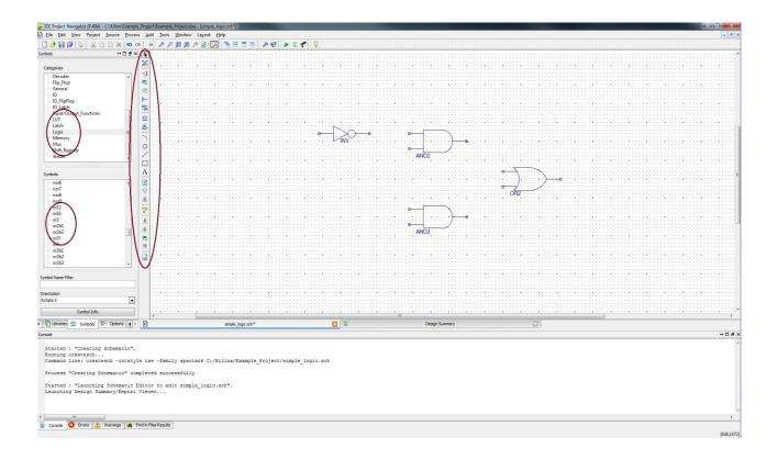
5. Use the wiring tool to wire up the components. It is in the tool bar and looks like a red line and a pencil. You could also use **Add** →**Wire** from the menu. I'm using the following components (from the **Logic** category) in this example:
