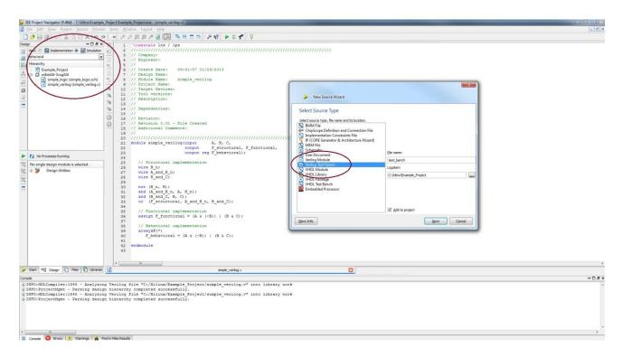
2. Click NEXT and choose which design you want to associate the test bench with. This is very important as you will have multiple modules or schematics in the future and you need to be sure which design will be going under test using the test bench. In this case I will just choose the "simple\_verilog" module to be tested. The procedure for testing the schematic version is exactly the same, you just have to choose the appropriate source to be associated with the test bench.
