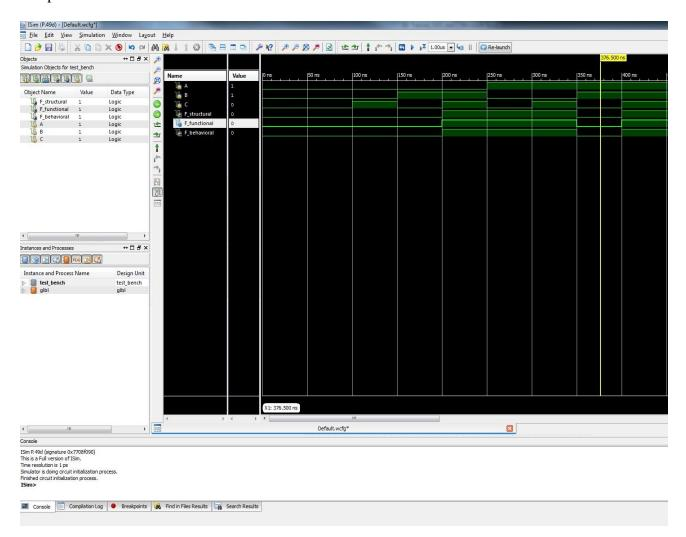
It is good to observe the other capabilities of your simulation windows. The console is where all of the simulator messages will be printed. Look for errors or warning about your design.
