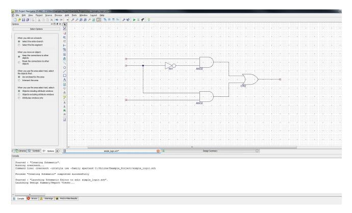
6. Now place **I/O Markers** to the inputs and outputs. I've used the **I/O Marker** widget that looks like two little labels. You can also use the **Add** → **I/O Marker** command from the menu. Click on the endpoints of the wire to add the marker.
