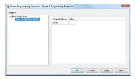
e. All that is left is to right click on the green chip icon with the Xilinx logo in the main pane and click **Program**. After the communication bar finishes, your design is programmed to the Nexys 3 FPGA board.
