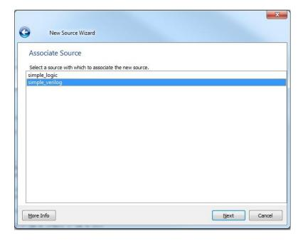
3. Click NEXT and after observing the summary click FINISH. Now you'll get a new piece of Verilog code generated for you. This Verilog code instantiates the "simple\_verilog" module as the UUT, and includes some other stuff related to how the UUT is connected to the testbench. It looks like this:
