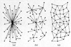
Fig. 1—(a) Centralized. (b) Decentralized. (c) Distributed networks
