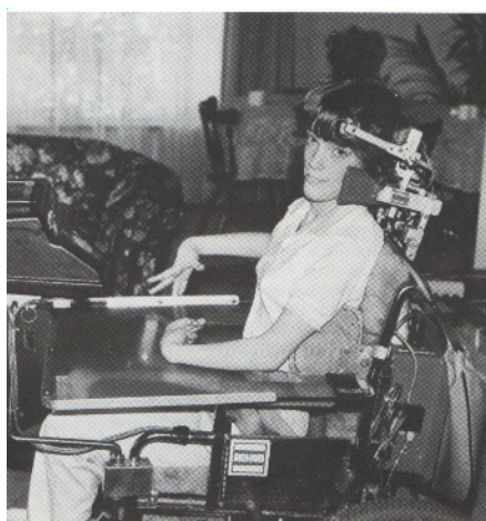
Kris Rytter with her Alternative Communication System. Whatever message Kris enters in Morse code is displayed on the readout or spoken by the speech synthesizer located in the device mounted on the front of the wheelchair.
