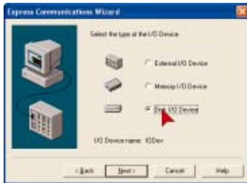
*A Disk I/O device emulates an external I/O Device such as PLC/RTU/DCS etc. A file on the hard drive is used to store an image of the variables. The file format is determined by the protocol being used. This is a great way to test your projects if you don't have an external I/O Device available. Memory I/O devices are the same, except they are stored in RAM and are therefore volatile.*
