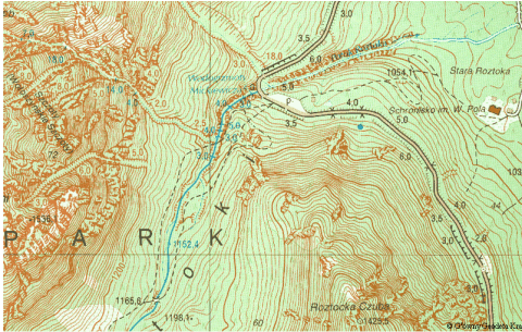
Figure: Contour lines join points of equal elevation above sea level
