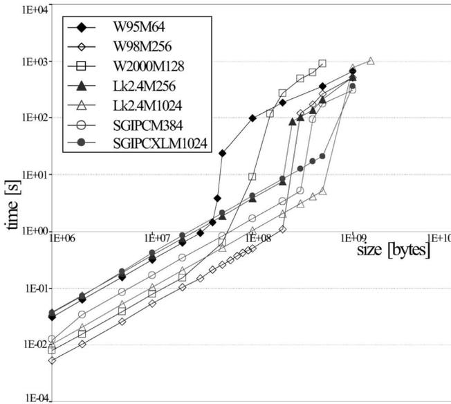
Fig. 1. Processing time of a simple search for a pattern in a linear array versus array size. In the legend,  $W_x$  denotes Windows version  $x$ , Lk2.4 denotes Linux with kernel version 2.4, SGIPC—SGI Power Challenge, SGIPCXL—SGI Power Challenge XL,  $M_y$  denotes core memory size  $y$  MB.
