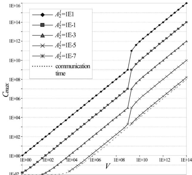
Fig. 6. Processing time versus  $V$  for various  $A_2^l$  and fixed  $swp$ ,  $A_2^h/A_2^l$ .
