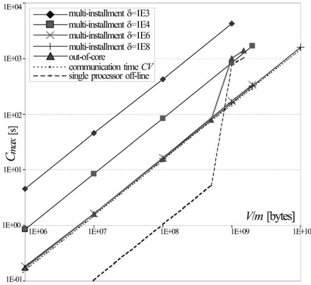
Fig. 11. Processing time versus  $\frac{V}{m}$  for multiinstallment and out-of-core computations on a cluster of Linux PC computers.
