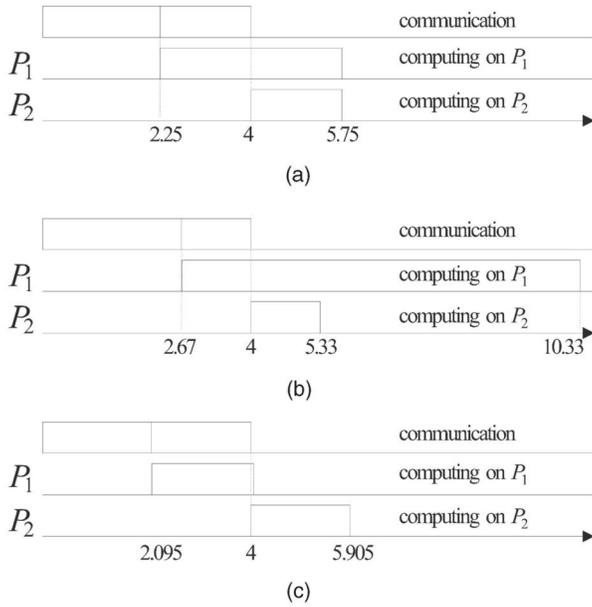
Fig. 3. Schedules for load distributions calculated assuming (a) hierarchical model of the memory, (b) computing in the core memory only, and (c) computing out-of-core only.
