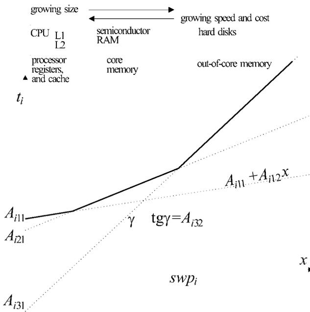
Fig. 2. Memory hierarchy diagram and a piecewise linear dependence of processing time on the size of the load.
