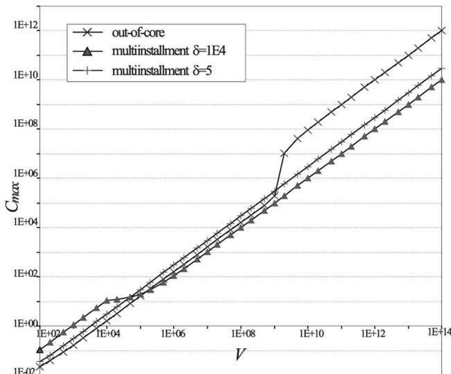
Fig. 10. Processing time versus  $V$  for multiinstallment and out-of-core computations.
