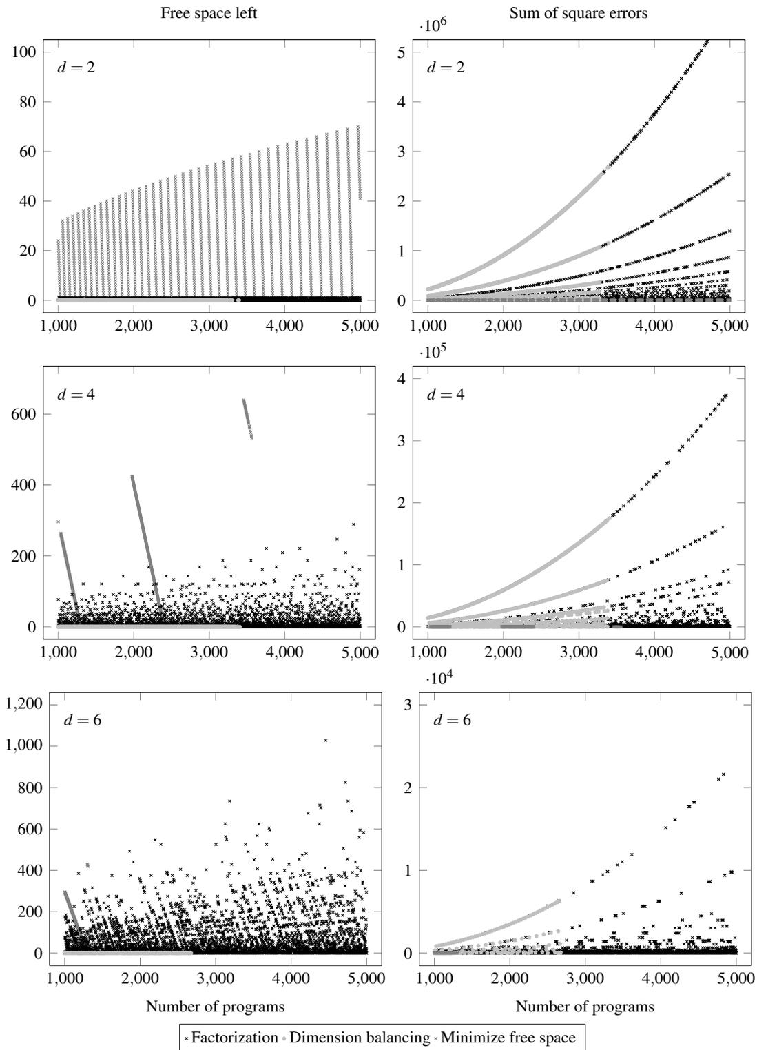
FIGURE 5.1: Comparison of hyperrectangle shape optimization methods: factorization, free space minimization and dimension balancing. The left column shows free space characteristics of each method, the right one refers to the sum of square errors between generated dimensions and optimal hypercube dimension size  $\sqrt[d]{|S|}$ , which usually is not integral value. Each row represents different dimensionality  $d \in \{2, 4, 6\}$  of the space.
