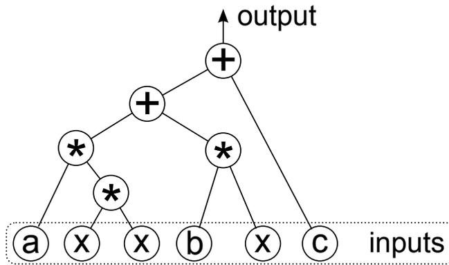
FIGURE 2.1: Example genome in canonical Genetic Programming. The tree in the picture represents function  $ax^2 + bx + c$ , where  $x$  is independent variable (function argument) and  $a, b, c$  are constants.
