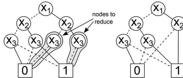
FIGURE 4.2: Binary decision diagram for expression  $f = \neg x_1 \neg x_2 \neg x_3 \vee x_1 x_2 \vee x_2 x_3$ . The dotted lines represent decision “0”, solid lines indicate decision “1”. Left: unreduced binary decision diagram, right: reduced ordered binary decision diagram.
