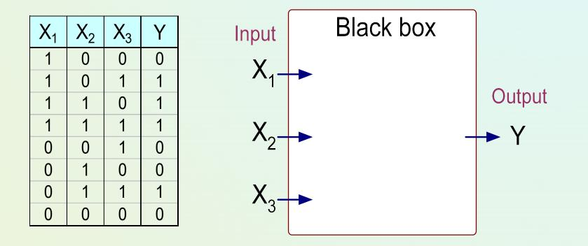
Output Y is 1 if at least two of the three inputs are equal to 1.
