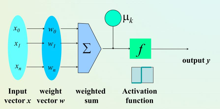
The *n*-dimensional input vector *x* is mapped into variable *y* by means of the scalar product and a nonlinear function mapping
