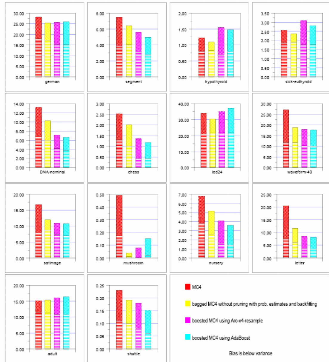
Figure 9. The bias and variance decomposition for MC4, backfit-p-Bagging, Arc-x4-resample, and AdaBoost. The boosting methods (Arc-x4 and AdaBoost) are able to reduce the bias over Bagging in some cases (e.g., DNA, chess, nursery, letter, shuttle). However, they also increase the variance (e.g., hypothyroid, sick-euthyroid, LED-24, mushroom, and adult).
