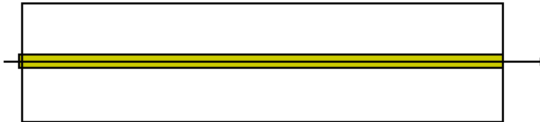
(b) Single-mode fiber: only direct path propagates in fiber
