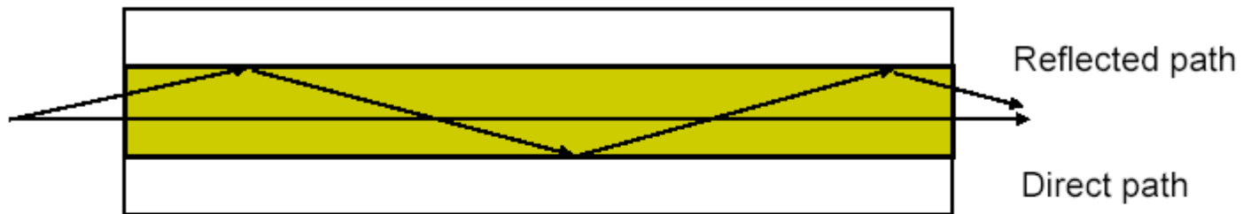
(a) Multimode fiber: multiple rays follow different paths
