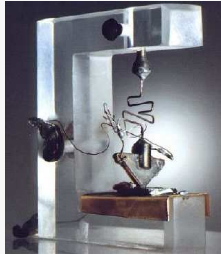
Prototyp tranzystora Bell Labs, USA, 1947
