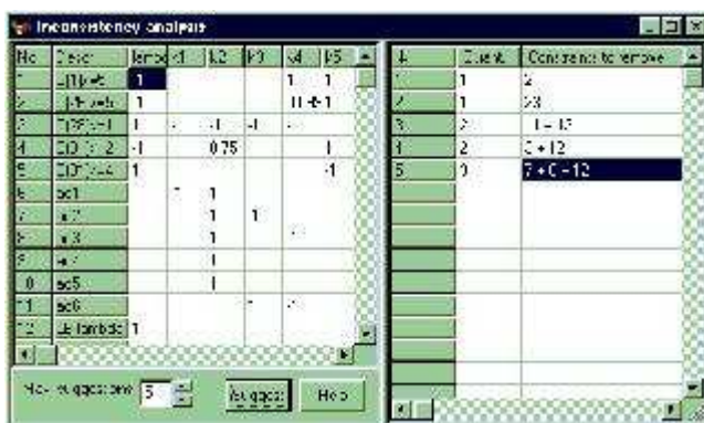
Figure 2. Given an inconsistent system of constraints (on the left), IRIS suggests five alternative ways to restore the consistency by removing constraints. The first suggestion is to remove constraint no. 2; the fifth suggestion is to remove constraints no. 7, 8, and 12.
