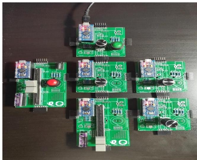
**Figure 5.** An example of a modular physical interface used to control interactive multiobjective optimization methods. Top: rotating knob with green button. Middle: slider with red button (left), rotating knob (center), rotating knob (right). Bottom: slider (center), rotating knob (right). The layout of the interface may be changed by connecting modules to each other using the pins and sockets present on the sides of each module.
